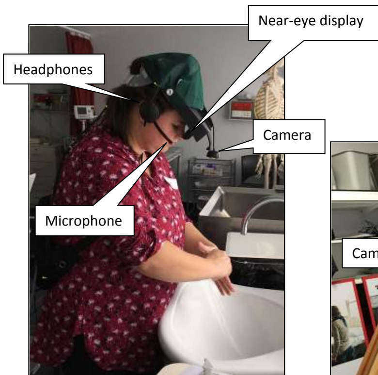
Figure 2. The student's unit. (HMD microphone, headphones, camera and near-eye display).
